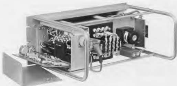
Figure 3. Rear view of a regulator with dust cover removed and etched board swung out for access to components and wiring.
